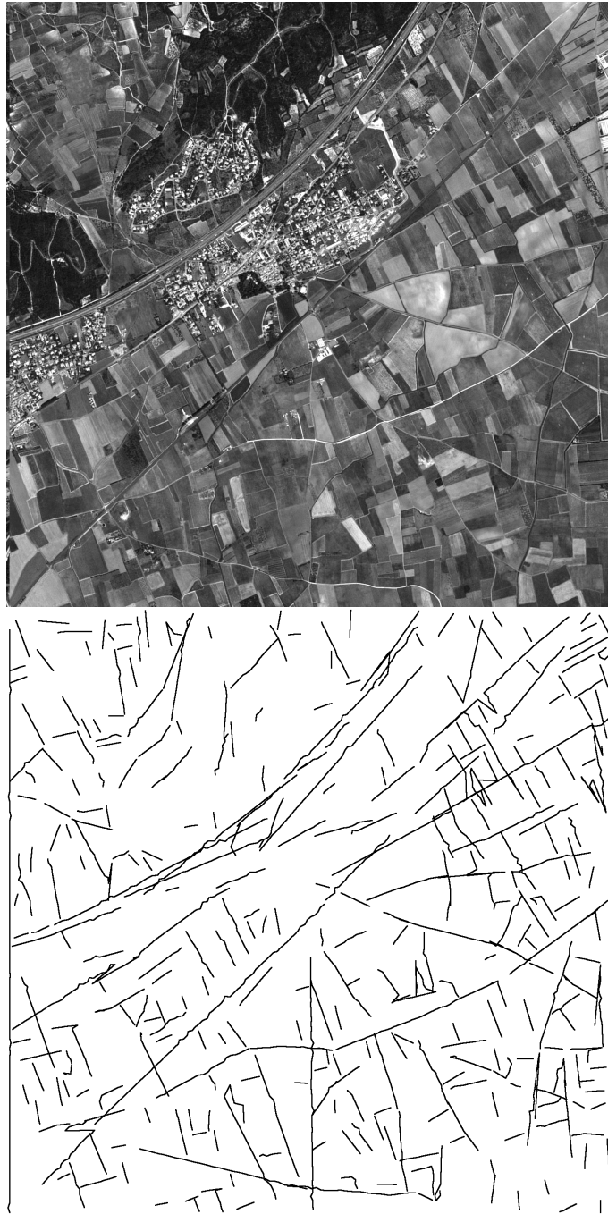
Figure 3.16: Example of road network detection: original image on top, detected roads on bottom.
