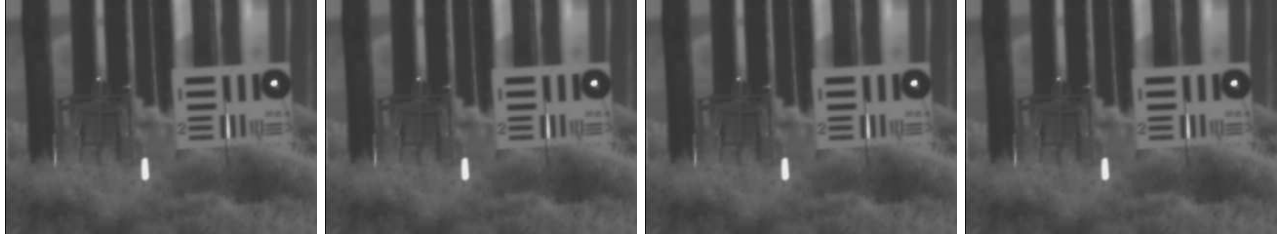
Figure 8. Restored images obtained from the different regularizers (30 input frames). From left to right: NLTV, TV, Framelet, Curvelet.
