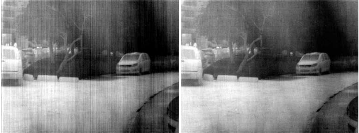
Figure 10. On the left : a real raw image taken by an infrared camera. On the right the result of ADMIRE.
