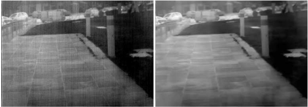
Figure 13. On the left : a real raw image taken by an infrared camera. On the right the result of ADMIRE.
