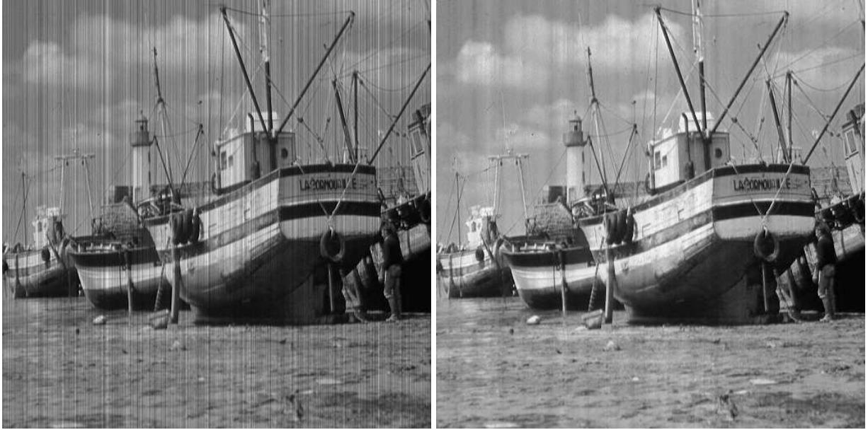
Figure 6. On the left : an image with a strong simulated non linear non uniformity. On the right : the image processed by the proposed algorithm. RMSE = 9.6629 , RMSE^{CI} = 5.7314 .
