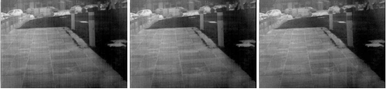
Figure 5. On the left : a real raw image produced by an infrared camera. Middle : the result of the algorithm with the parameter s = 1 . On the right with s = 7.5 . For example, focusing on a zone in the middle of the image the image with s = 7.5 is nicer but, the zone below poles is bad. On the other hand in the image processed with s = 1 the zone in the middle is still corrupted by the non uniformity. Thus, a fixed s parameter for the whole image will not lead to the best quality possible everywhere.
