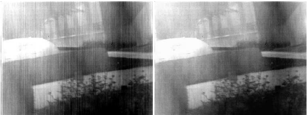
Figure 12. On the left : a real raw image taken by an infrared camera. On the right the result of ADMIRE.
