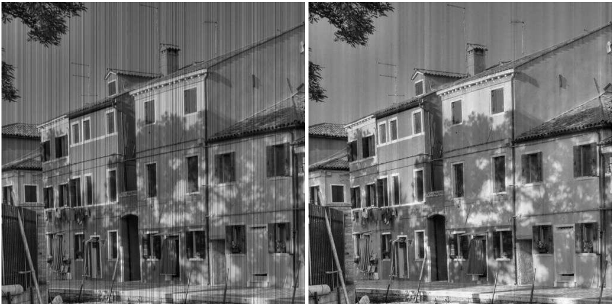
Figure 7. On the left : an image with a strong simulated non linear non uniformity. On the right : the image processed by the proposed algorithm. RMSE = 8.7100 , RMSE^{CI} = 7.3411 .
