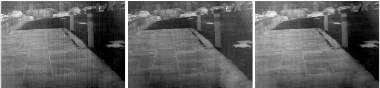
Figure 9. On the left : a real raw image of an outdoor scene taken by an infrared camera. Middle : the total variation based method. Notice the artefacts created bellow the poles. On the right the proposed method (we deactivate the DCT denoising to provide a fair comparison).
