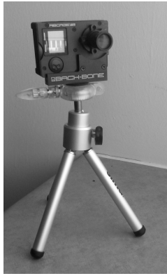
Fig. 1: RibCage Air Modified GoPro Hero 4 Black camera with a 25mm f/2.0 14d HFOV 3MP lens on its tripod.
