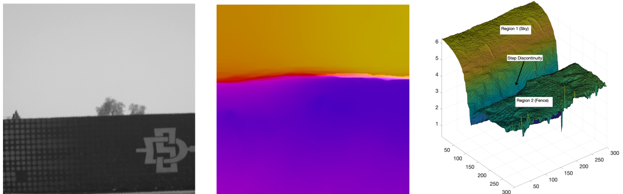
Figure 14: Depiction of the step discontinuity in the magnitude of the optical flow corresponding to an instantaneous change in depth \mathcal{Z} . Frame 90 from Field4 (left) is presented with a colored depiction of the optical flow (center) and the magnitude of the optical flow (right).
